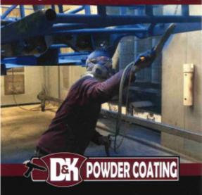
applied electrostatically and cured under heat. Powder coating creates a long-lasting finish that is substantially stronger than conventional paint. Powder coating is a solvent-free, environmentally friendly finish that virtually eliminates air and water pollution. Powder coating is one of the most durable and least expensive paint finishes available today!
